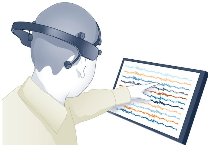
**Fig. 1 | An EEG recording in 2024.** An illustration of a young participant wearing a modern wireless headset recording EEG outside of the laboratory in a school classroom setting in Bradford, UK, in 2024. The signal displayed on the screen, repeated across rows, is an adaptation of an early recording taken by Hans Berger from his son Klaus<sup>1</sup> a century earlier, showing sinusoidal 10-Hz activity, which he referred to as the ‘alpha rhythm’.
